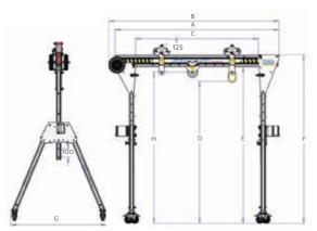
Frames easily fold onto beam forming compact, stowable unit. Fits into a typical service van.
