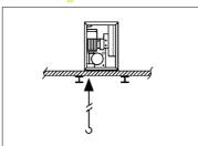
If the hole is not big enough for the rope hook to pass through, position the TIRAK mobile winch and pass the wire rope through the hole and then into
