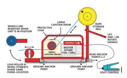
NOTE: WHEELS MUST BE REMOVED WHEN MACHINE IS IN POSITION THIS WILL GROUND THE MACHINE SUITABLE FOR ANCHORAGE AND ENABLES THE LEAD ROLLER TO UTILISE THE SAME FIXINGS.
