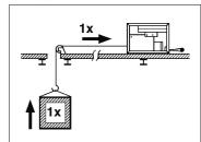
To lift: anchor the TIRAK mobile winch to a suitable point and pass the wire rope around one or more return pulleys.
