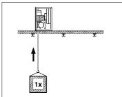
If the pull is through an opening in the wall or ceiling capable of taking the load, simply site the winch by or above the hole.
