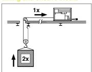
If the effective power is not enough increase the capacity using a set of multiple sheave blocks.
